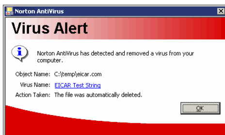
Figure 13-12: Using the EICAR test string to test antivirus software.
