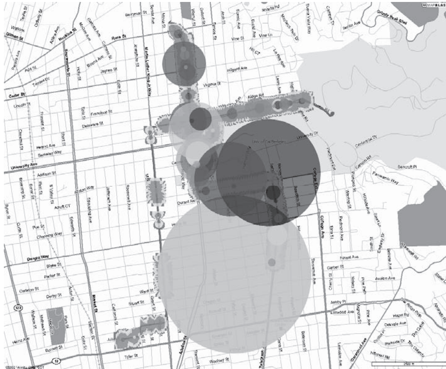
Figure 2-10 Kismet can be used while wardriving to develop wireless network maps.
