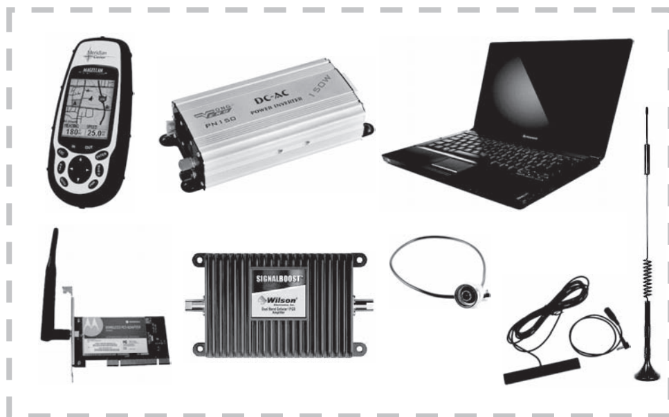
Figure 2-19 Man-in-the-middle attacks require specific hardware as well as software.
