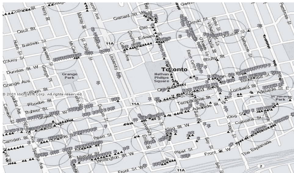
Figure 2-7 Wardriving enables the user to make maps of WLANs in a geographic area.
